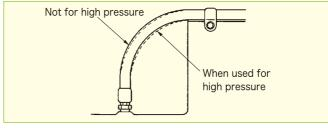
When the hose has inner pressure by fluid, hose length will slightly change. But do not fix the bending portion to suppress the change.
