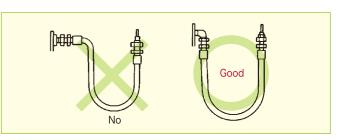
By applying elbow, please avoid extreme torsion or bending.
