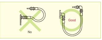
When using the hose in minimum bending radius, apply elbow as shown in the sketch to avoid sharp bending.
