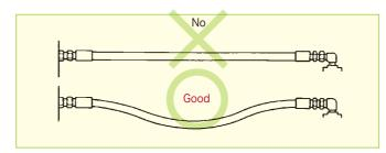
When the hose is used for high pressure, length will change in range of +2% and -4%. So, it must have sufficient looseness.
